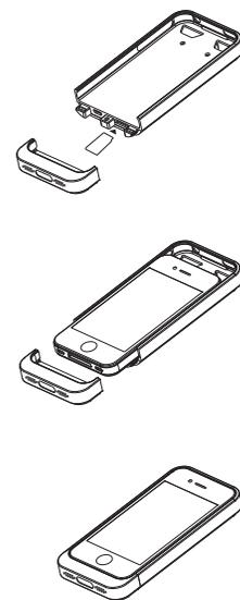
1. With the gold contacts facing downwards insert memory card in the slot until it clicks into place.
