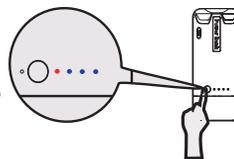
( Please note a blue LED will blink when battery is lower than 5%, the unit will not be functional, charge the battery immediately. )
