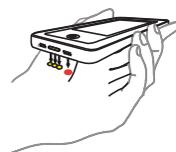
3. You can discreetly check on the recording status by holding the unit in hand, with a steady red LED turned on it means a recording is taking place and the other three blue LED are the battery capacity.
