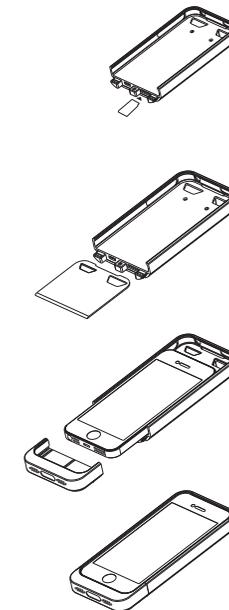
1. With the gold contacts facing downwards insert memory card in the slot until it clicks into place.
