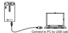
1. With the unit powered off, connect the supplier USB cable to the USB port on the base of the device.
